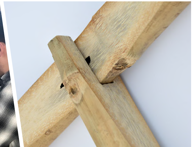
Detail of joined milled bamboo slabs. (below) Courtesy of Virginia Tech.
